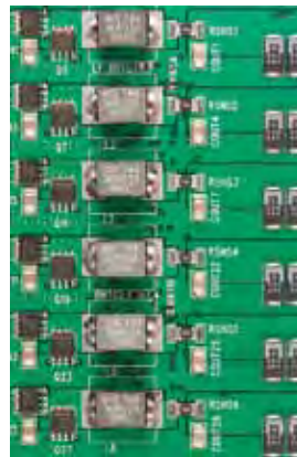
V_{IN} = 7V to 14V V_{OUT} = 1.5V@120A 6-Phase Design with 2 LTC3829 ICs
