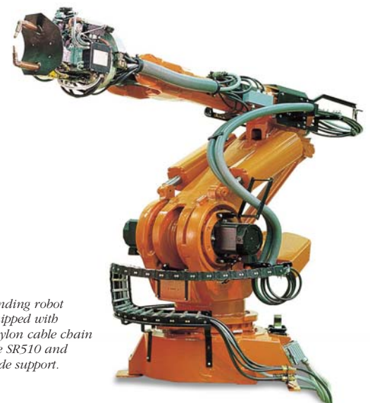
Circular nylon chains on welding robots.
