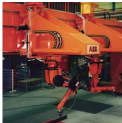
Welding robot equipped with nylon chains.
