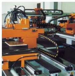
Machine tools equipped with Heavy series cable chains.
