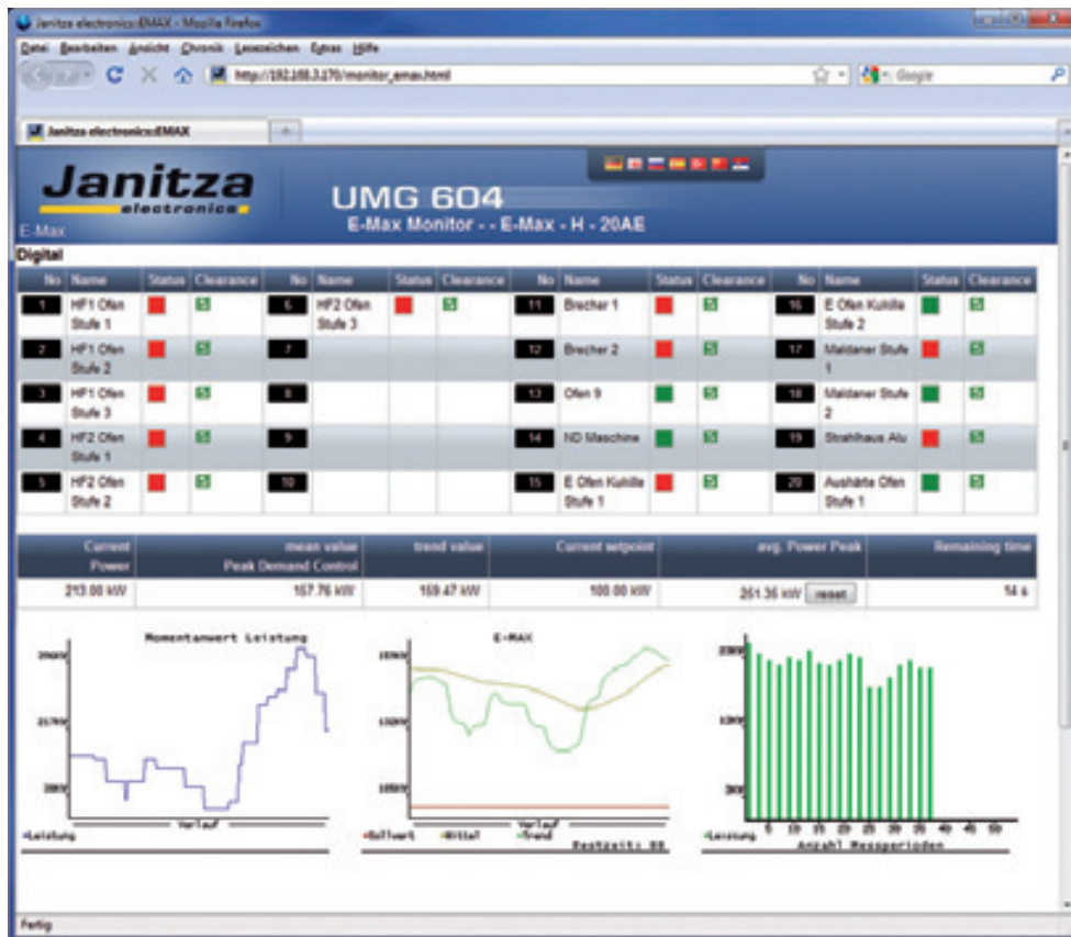
Status display of Emax measured quantities and status of the current switch-off actions, status of the release (feedback as to whether a load is on/off) via the device homepage.
