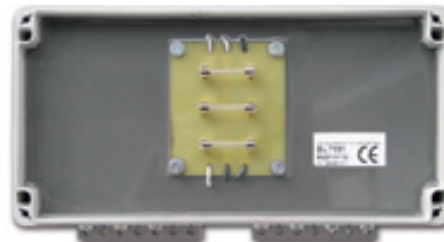
Diag.: Voltage transformer without cover with fuses
