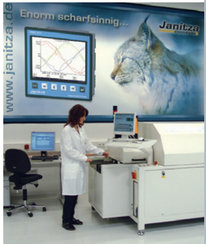
Reflow soldering machine in the PQM device production
