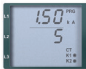
Programming Current transformer
