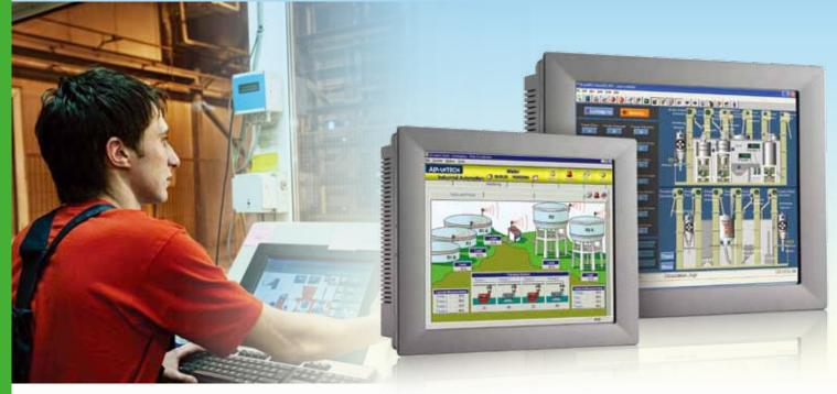
With energy saving LED backlight LCD display, TPC-71H series is designed with the low power consumption Intel<sup>®</sup> Atom<sup>™</sup> D525 processor 1.8GHz as its core; fanless but with powerful kernel. With PCI-e expansion and DIO control support, TPC-71H series are designed for automation applications as a control panel solution in a variety of industries
