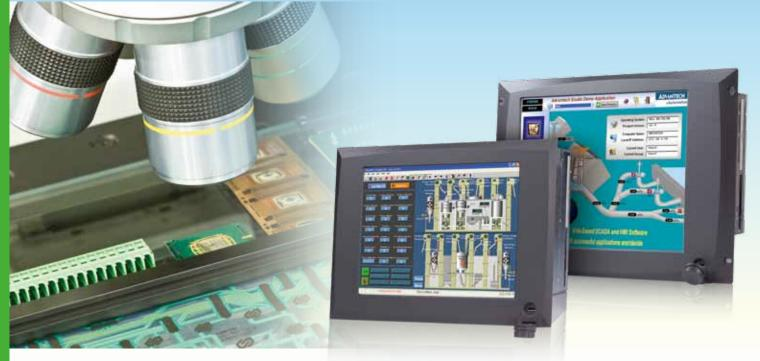
With latest Intel<sup>®</sup> Core<sup>™</sup> i7 mobile processor, IPPC-9000 series provides high computing performance at the same time supports intelligent iManager with value-added APIs & runtime OS QNX. In addition, design with die-cast bezel and stainless steel housing makes it extremely rugged but compact. Positioned as a rugged & intelligent panel PC, IPPC-9000 series is suitable for monitor and control management or even complicated applications like surveillance systems.
