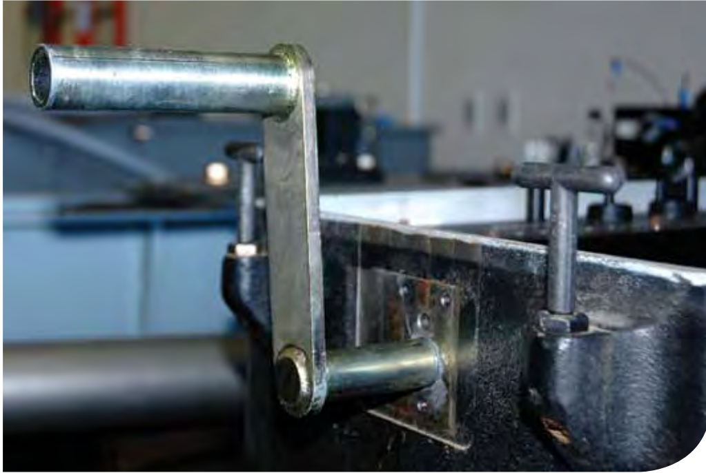
GM4000A™ Switch Machine Hand Crank
