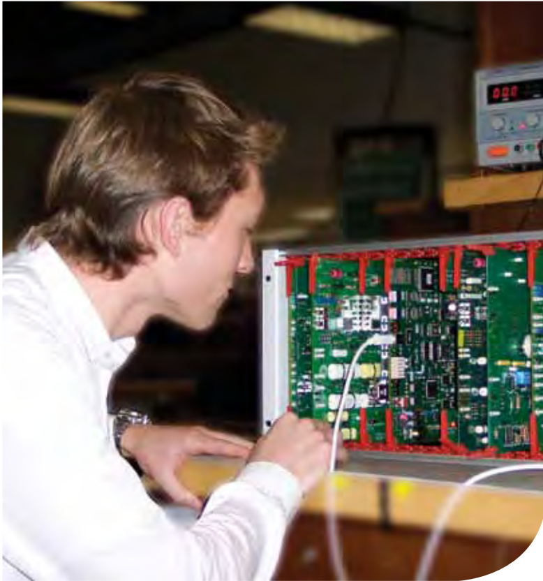
AF Track Circuit being tested at the Rochester, NY facility
