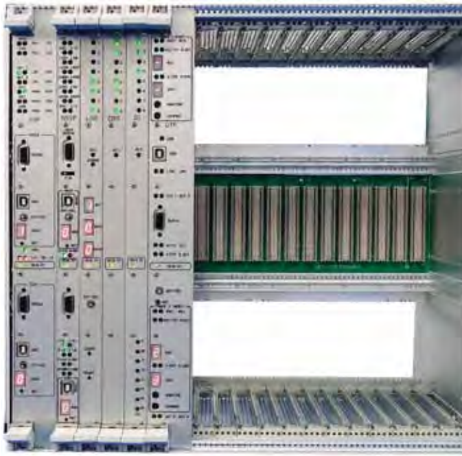
iVPI 21-Slot Main Chassis
