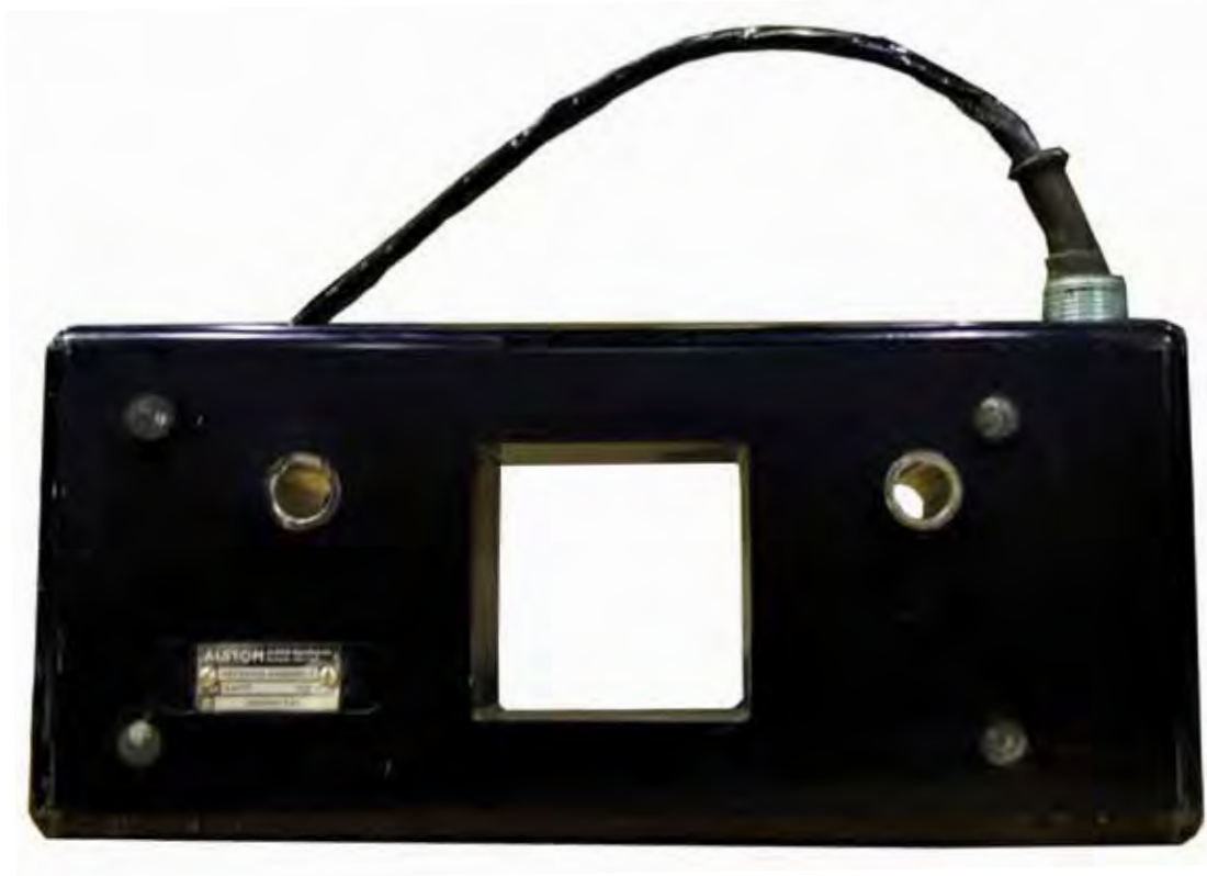
Typical Cab Signaling Receiver Coil
