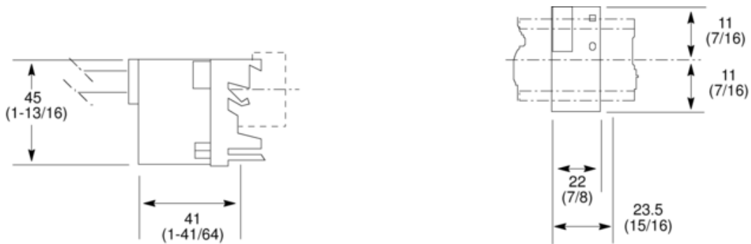
Timer With DIN Rail Mounting Adapter on 35 mm DIN Rail Cat. No. 196-MT Timer With DIN Rail Mounting Adapter on 35 mm DIN Rail Cat. No. 196-MT
