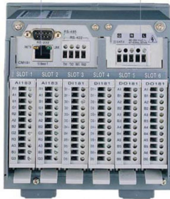
6 SLOTS for Plug & play I/O cards, maximum 18 analog input or mixed with analog & digital I/O cards
