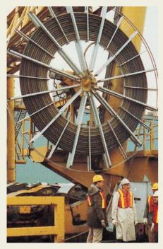
A large, high speed Cavotec Specimas cable reel mounted on a coil handler running at 180 m/minute.
