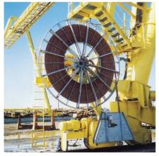
A Cavotec Specimas cable reel working at ± 200 m/min on a P&H log-handling crane for Federal Paper Board, in Augusta USA.
