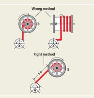
Figure 3. Transfer of cable from original delivery drum A to the cable winding reel B.
