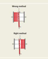
Figure 4. Winding of cable onto multi-spire reel.
