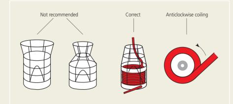
Figure 1. Shape of the basket and direction of coiling.
