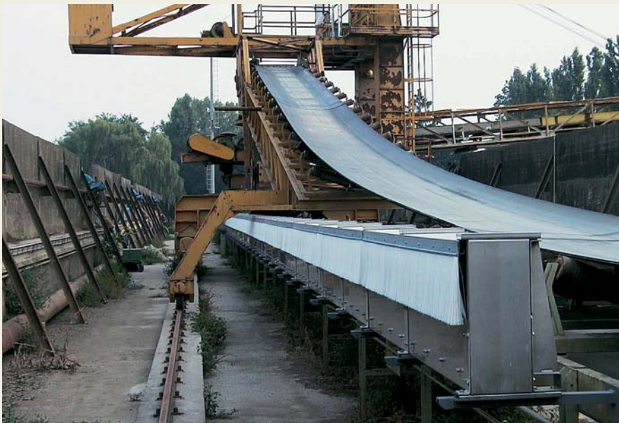
In action at a sugar plant. This nylon chain operates in a fully enclosed cover which prevents dust from entering the chain pathway. The passage of the towing arm is fully protected by brushes.
