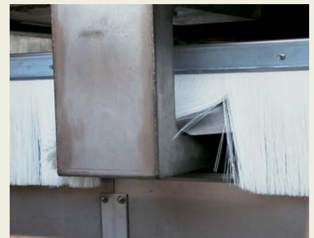
In action at a sugar plant. This nylon chain operates in a fully enclosed cover which prevents dust from entering the chain pathway. The passage of the towing arm is fully protected by brushes.
