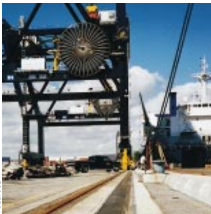
Cavotec Specimas cable reels with "pull and store" and Panzerbelt® in operation at Everglades Terminal, USA.
