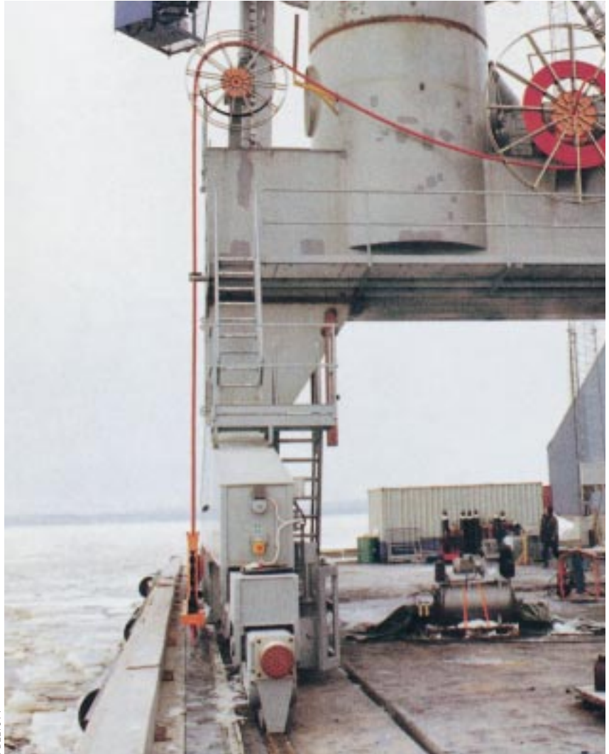
Halmstad, Sweden, Cavotec Specimas Panzerbelt® and reel working at minus 35°C
