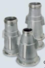
Where larger, stiffer cables are involved, Cavotec Connectors offers a choice of longer, larger-entrance end-bells. Two sizes are available that can accommodate cable sizes through 4 1/4" O.D., with clamps to fit cables 1 1/4" - 4 1/4" O.D. Where end-bell
