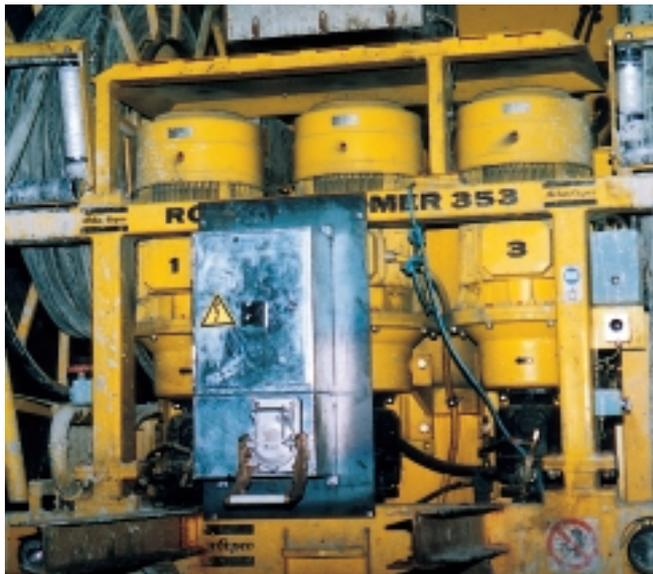
This photograph shows a tunnelling site in Stockholm where the excavation work is carried out by means of an Atlas Copco drilling rig with a Cavotec Connectors panel for power supply to a shotcrete machine.
