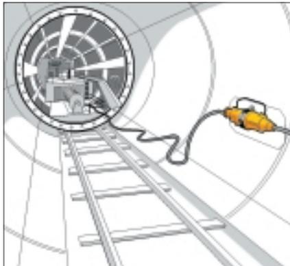
*A tunnelling application for power feed to a full-face drilling machine*
