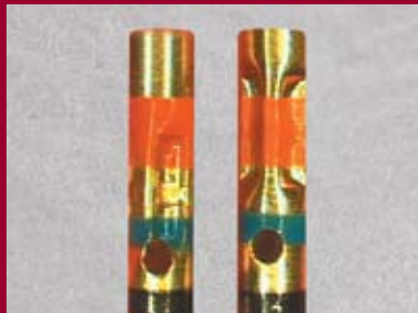
Example of a poor crimp showing deformation of the inspection hole against a correct example. This is caused by incorrect tool settings.
