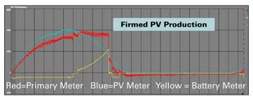
Figure 2. Power Shaping of PV Array<sup>1</sup>
