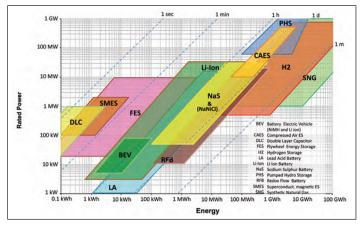
Figure 4. Energy Storage System Ratings<sup>3</sup>
