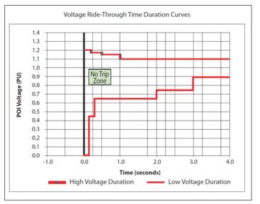
Figure 3. NERC Requirements for Voltage Ride-Through<sup>2</sup>
