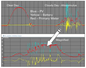
Figure 1. Solar Power During a Cloudy Day, with Energy Storage Reducing Power Rate of Change to the Grid<sup>1</sup>
