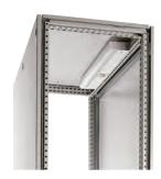
**Description:** Fluorescent lamp equipped with switch electronic starter integrated socket and a protection cap. A male GST 18/ 3 connector is provided for connection to the power on one side and by a pass-through circuit to a female connector allows a further connection on the other side. An additional connector ST 17/2 allows the activation of the lamp by a door switch. Power: Standard socket:120/230 V/ 50/60Hz / 16A Schuko. Other country specific sockets available on request.
