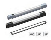
Description: It's compact design makes it suitable for mounting in almost any enclosure or rack. Supplied including three integrated fixing methods e.g. magnet, screw and snapin and a connection cable. Provided with a protection cap, electronic quick start and 3-way switch (on/off, door switch, permanent light). An integrated socket permits operation by an optional door switch.
