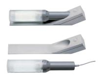
Description: Energy saving lamp for fixed use or with addition of the accessory LTHC as removable hand-lamp for more precise illumination. Self-adhesive or screw fixing support, provided with push button on/off switch.
