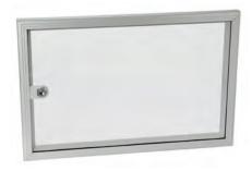
Description: To replace the steel door. Can be used in combination with swing frame, modular chassis or inner door. The double-bit 3mm lock can be replaced by any optional insert or handle. It increases the enclosure depth in 10mm (ADA) or 35mm (ADAB). Can also be used as a viewing window when used in combination with mounting kit ADAMK/ ADABMK.
