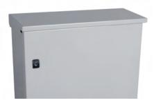
**Description:** To be fitted as an outdoor shelter on single mounted enclosures. The roof is slightly sloped and has a dripstrip. Machining is required. It increases the enclosure dimension in H:60mm, D:20mm and W:20mm
