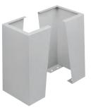
**Description:** Floor stands for floor mounting to give a suitable operation height. Available for 300 and 400mm depth enclosures with  $W \ge 400$ mm. 300 or 450 mm high are available. Machining is required
