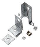
**Description:** Mounted on to the back of the ACM or CMV modular system frames, allowing the fixing of the AMM mounting plate. The mounting plate is adjustable in depth between 60mm and 150mm from the front covers. **Material:** 2mm galvanized steel.
