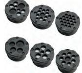
Description: Round plastic cable entry for a fast, economical and tool-free incoming of cables and/or pneumatic conduits inside the enclosure. Integrated seal. For snap-in mounting. Snap-in system works at wall thicknesses of 1.5 to 2.0mm. Installation height: 9mm outside, and 24-25 inside. Material: Polyamide, and the seal is made of NBR/EPDM, halogen free. Temperature resistance: -30°C to +90°C Flammability: VO according to UL94 Finish: Black Protection: IP 65
