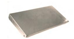
**Description:** To be fitted as extra protection on single mounted enclosures. The roof is slightly sloped and has a dripstrip. Machining is required. **Material:** AISI 304 / AISI 316L pre-grained stainless steel **Finish:** 240s pre-grained stainless steel (average 0.5 micron) **Pack quantity:** 1 rain hood with mounting material.
