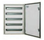
Description: Used for easy mounting of DIN-rail components with a maximum height of 68mm. Distance between rows 125mm. If required, the standard enclosure door can be replaced with a glazed door. Usable depth between front cover and external door: 35mm. Adjustable depth position with AMG accessory. In stainless steel enclosure machining is required. Material: DIN-rails PP0735 made of 1.20mm galvanized steel, vertical profiles 1.5mm mild steel, and front cover 1.5mm mild steel.
