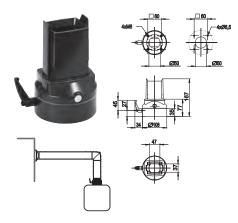
Description: Coupling component for SM system, angle of rotation 300 degrees with stop.
