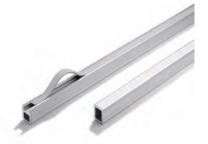
**Description:** The arm section profile is available with an open cable duct or completely closed. In the open profile the plastic cover can be easily pulled out and fitted back into place. **Material:** Extruded aluminium profile. Plastic cover in the open profile made from EPDM.
