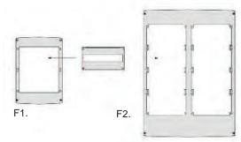
Description: Frame to be covered with individual cover plates UICP. For enclosures 600 and 800 mm wide it has 2 columns.
