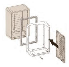
Description: Increases the standard depth (320mm) of the enclosure up to 640mm. When this accessory is used the rain hood cannot be used.
