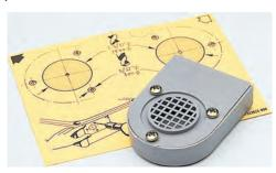
Description: Two air vents must be mounted per enclosure to ensure sufficient air circulation and prevent water condensation. Air vents are preferably mounted in the upper and lower part of the enclosure. Degree protection: IP 44.
