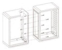
Description: Kit to allow vertical and/or lateral combinations. Machining is required.
