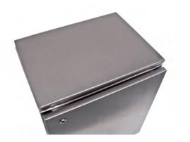
**Description:** Used to cover top openings of base, or desk units where hard wearing or corrosion resistance is required. **Material:** 2mm AISI 304 pre-grained stainless steel. **Finish:** 240s pre-grained stainless steel (average 0.5 micron) **Pack quantity:** 1 piece with mounting accessories.
