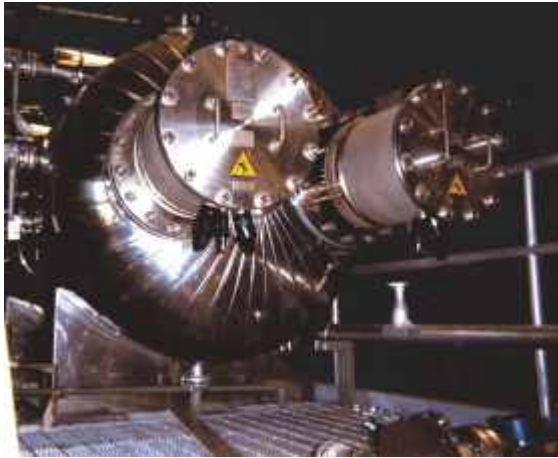
Process immersion heaters
