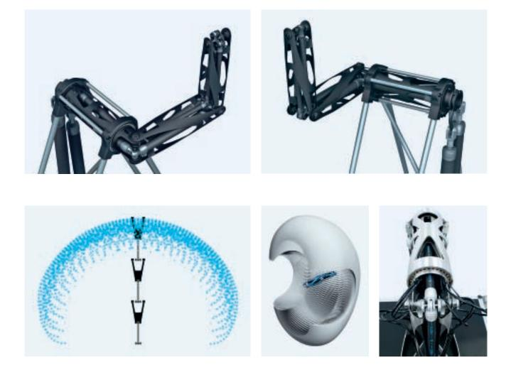
To attain optimum kinetics for the arm system, the standard muscles of Festo were modified in the following points: Specially shortened fork joints were designed, and the opposed bearings were devised as integrated press connections that ensure compressed air supply, self-centring and the required degree of rotation.
