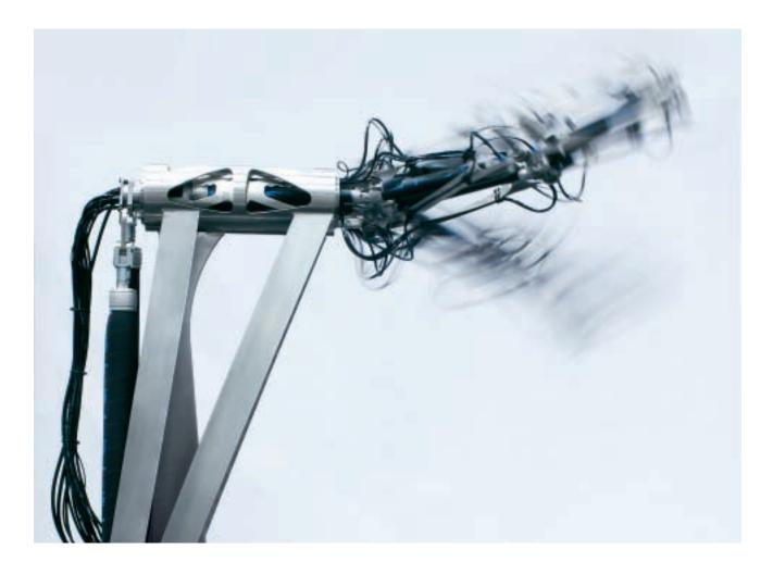
Biologically inspired by analyses of lobsters' and grasshoppers' legs and of human pointing gestures, a two-segmented arm with an external skeleton has been developed with movement patterns similar to those of a human. Powered by pneumatic muscles, "AirArm" catches drops of water.
