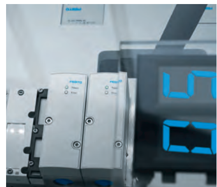
Pressure control in the pneumatic muscles: the VPPM valves
