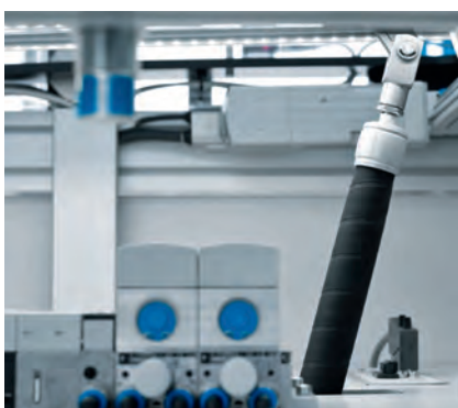
Tilting the field with compressed air: the DMSF-20 pneumatic muscles
