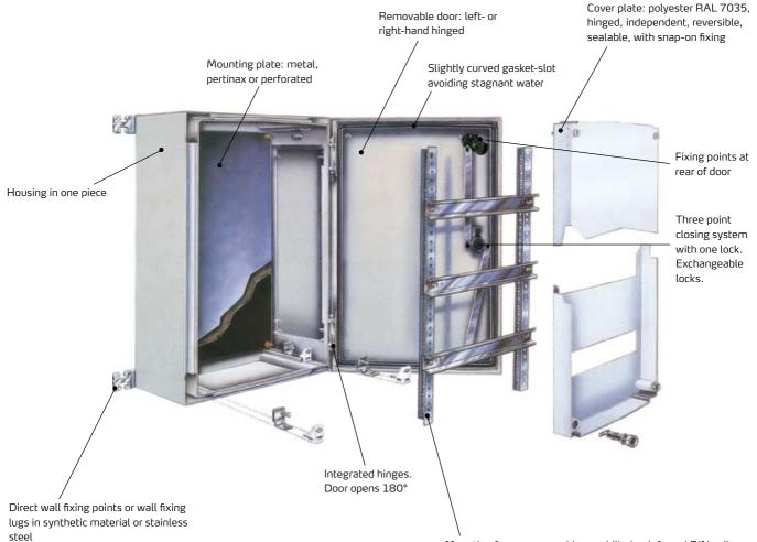
Mounting frame: removable, predrilled, reinforced DIN-rails
