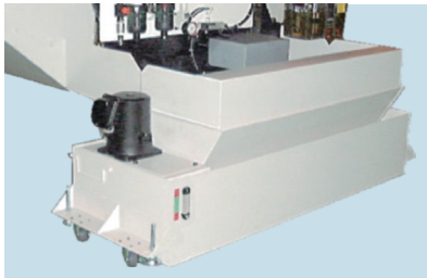
Coolant unit (tank)
