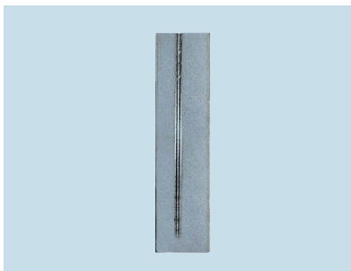
Deep hole drilling(section) Dia.3.3x96mm (Stainless)
