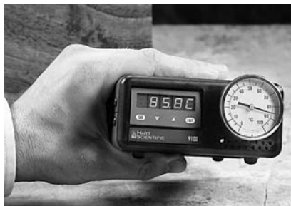
Handheld block calibrators have made industrial calibrations more portable.
