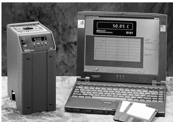
Includes an RS-232 port and free Windows control software (Interface- it ) to automate your dry-well.
