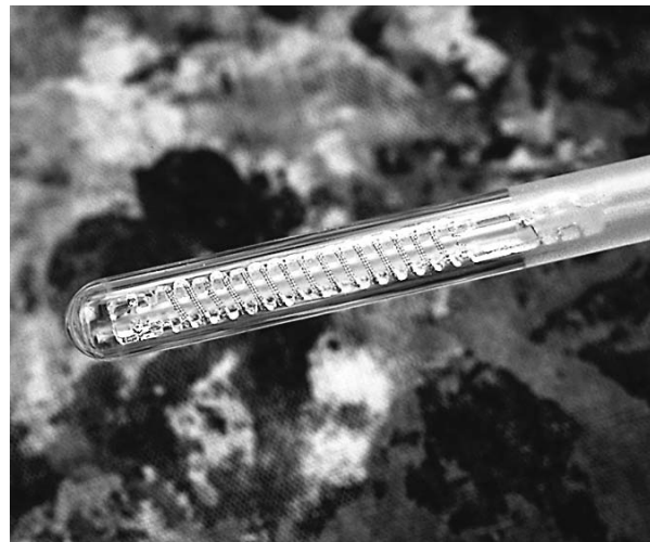
A close-up of a 25 \Omega spiral-wound helix SPRT element.
