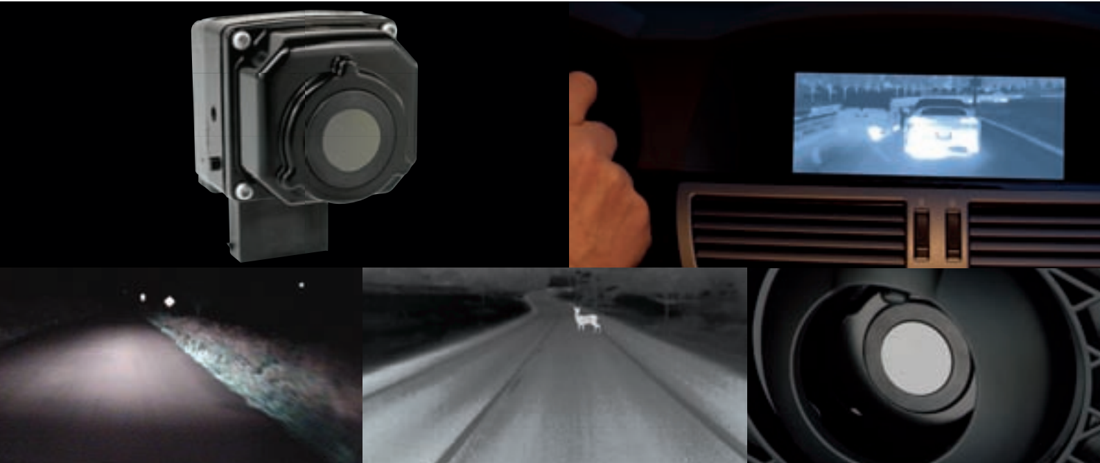
Clockwise, from upper left corner: FLIR PathFindIR, in-dash display, PathFindIR grill mount, deer crossing a road and visible light image showing that headlights haven't yet detected the deer.
