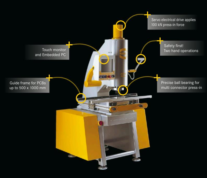
Outstanding flexibility, combined with the high press-in force capacity of the CPM *prestige* makes it suitable for any number of applications.
