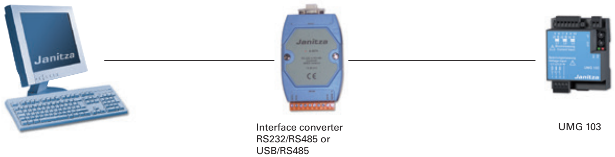
The connection of a UMG 103 to a PC using an interface converter
