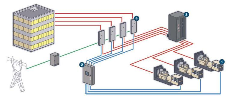
The KOHLER® Decision-Maker® Paralleling System (DPS) offers a truly integrated approach to generator paralleling. Each system includes generators, Decision-Maker 6000 controllers, a master control panel, power distribution switchboards with breakers and KOHLER automatic transfer switches.
