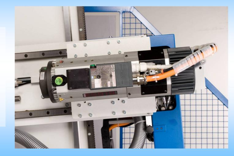
Hollow shaft spindle
