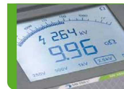
Large analogue / digital LCD with backlight
