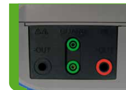
Guard terminal for connecting shielded test leads
