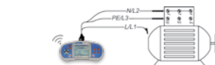
Test circuit for continuous resistance measurement
