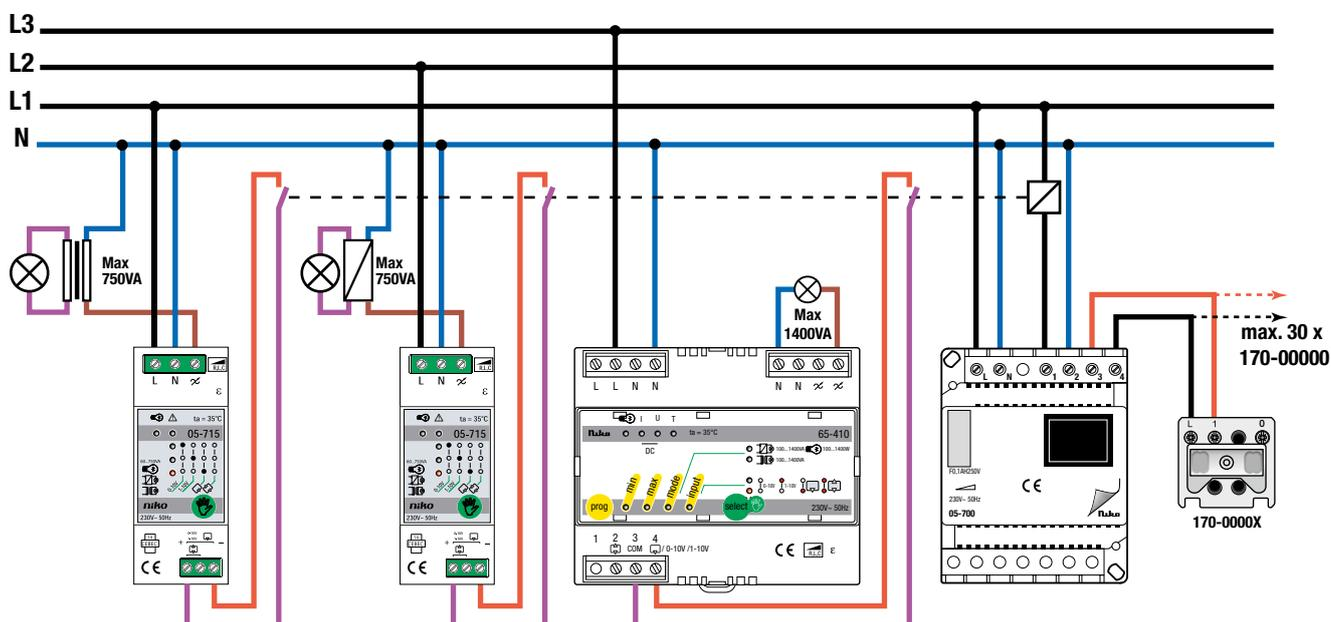
Control with 2 N.O. push buttons, 1 push button for on/dimming up and 1 push button for off/dimming down
