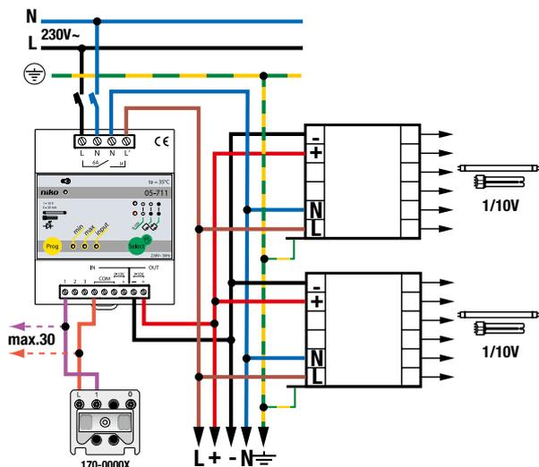
**Control with 2 N.O. push buttons, 1 push button for on/dimming up and 1 push button for off/dimming down, for fluorescent lighting**
