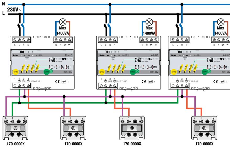
**Rotary switch control of different light circuits connected to a 3-phase mains voltage**
