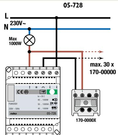
Control with push button 230V~, connected via a relay
