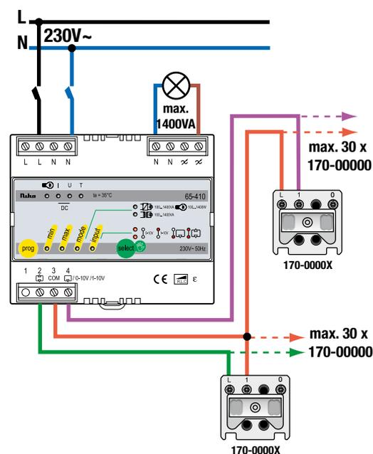
**Controlling different light circuits with separate dim function and central switch-off function by means of N.O. push buttons**
