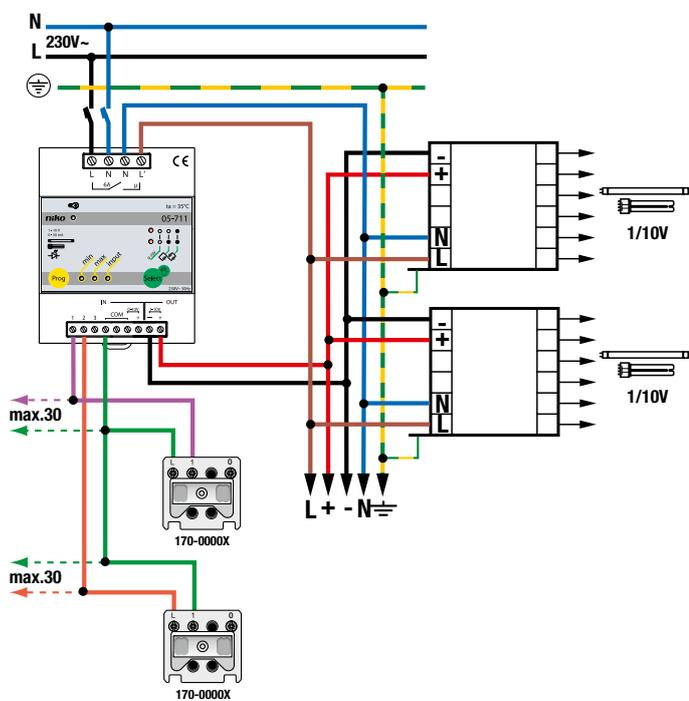
**Controlling different light circuits with separate dim function and central switch-off function by means of N.O. push buttons, for fluorescent lighting**
