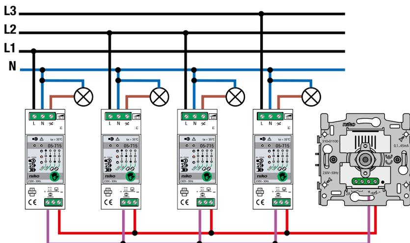
**Control with push button non-voltage, separately derived from the mains, for fluorescent lighting**
