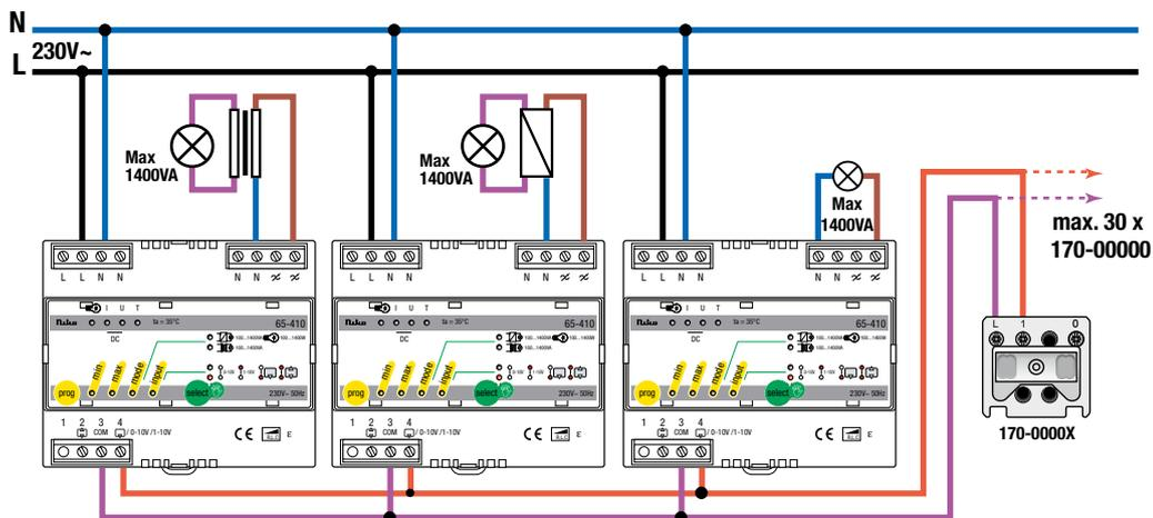
Simultaneously controlling different light circuits connected to a 3-phase mains voltage via a relay and control module 05-700
