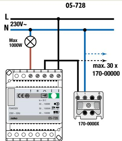
Control with push button 230V~, connected to phase
