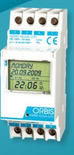
The ASTRO NOVA CITY is a time switch which controls the switching ON/OFF of any lighting circuit or installation according to the dawn and dusk of the area. The different areas are programmed using an easy text menu. The times are set using the main cities of your country and therefore you simply choose the city closest to you. The installation uses Din rail without the need of any external wiring out of the cabinet; also, it does not require any maintenance to maintain the accuracy.
