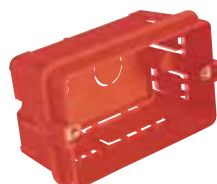
2175 Sacatola rettangolare in Tecnopolimero con 2 inserti metallici - Interasse fori 83,5mm - Dimensioni interne: 93x55x50mm - Confezione in termoretraibile Technopolymer rectangular box with two threaded metal parts - Distance between fixing centres 83,5mm - Inter- nal Sizes: 93x55x50mm - Wrapping in therm-retractile plastic
