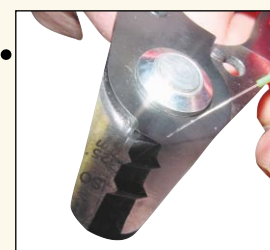
Abisolieren des Primär-Coatings stripping of primary coating
