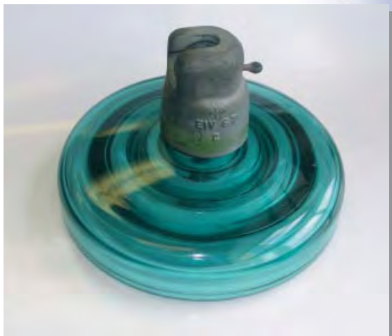
45 year old toughened glass insulator string in service on a 500 kV line.
