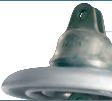
Suspension insulators are available for ball & socket or clevis-eye coupling. Standard caps are constructed of hot-dip galvanized malleable iron. Cotter keys for locking ball & socket and clevis pin connections are stainless steel.
