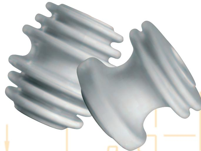
The umbrella type spreading porcelain shell or shed protects the leakage corrugations on the underside of the insulator from contamination and mechanical damage. The sheds are designed to provide optimum normal and protected leakage distance in relation to size and shape.
