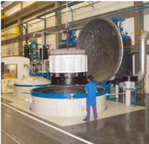
VPI System Diameter: 3.5 m Height: 6 m
