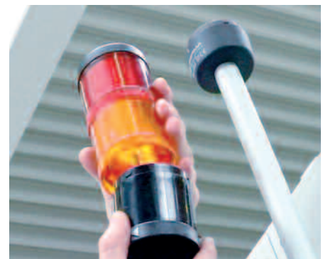
Simply fit the KombiSIGN reflect slave to the signal tower on the machine
