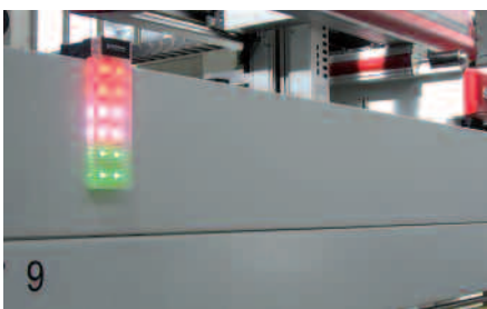
Tier-by-tier illumination of the lighting body
