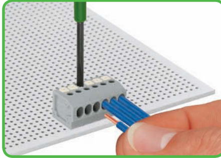
Inserting solid conductors by simply pushing them in. Inserting and removing fine-stranded conductors via push-buttons.
