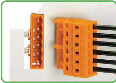
Panel feedthrough male header in large cutout. Coding using coding keys. Coding finger(s) opposite of coding key(s) must be broken off.
