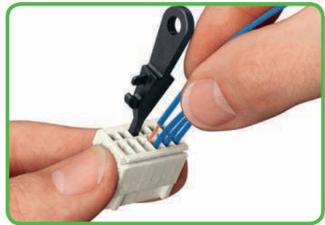
Conductor termination parallel to CAGE CLAMP® actuation
