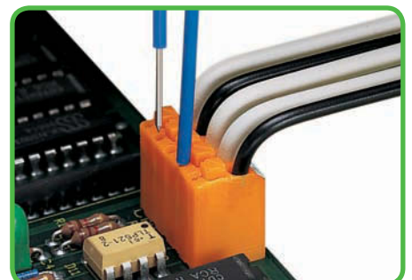
Testing with 1 mm Ø test pin.
