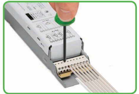
Removing a conductor by inserting disconnection tool into the operating slot and pulling it out.
