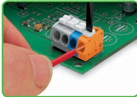
Inserting/removing fine-stranded conductor: Open clamping unit via push-button and insert stripped conductor until it hits backstop.
