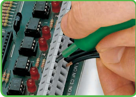
Inserting conductor via 3.5 mm screwdriver. Screwdriver actuation parallel to conductor entry.
