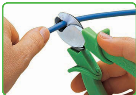
Cutting a conductor.
