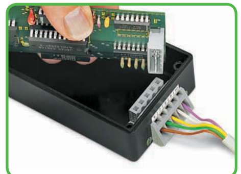
Angled female connector used as through-panel connector. Conductor entry and operation holes outside the housing. Panel thickness up to 2 mm/0.079 in.
