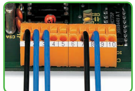
Pin center spacing can be maintained in an assembly.
