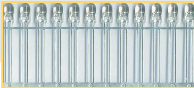
LEDs im Leadframe/ LED in a leadframe
