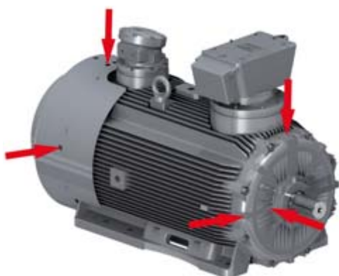
Figure 3.07 - Vibration monitoring directions
