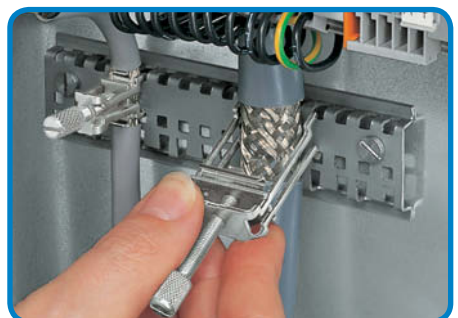
Tightening/releasing a shield (screen) clamping saddle. To attach the clamping saddle, tighten the knurled screw. To remove, unscrew until ratcheted mechanism is released, then slightly tip saddle and remove the clamping saddle.
