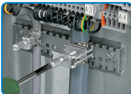
Tightening/releasing a shield (screen) clamping saddle. To attach the clamping saddle, tighten the knurled screw. To remove, unscrew until ratcheted mechanism is released, then slightly tip saddle and remove the clamping saddle.
