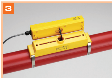
Connect power and sensors to electronic assembly
