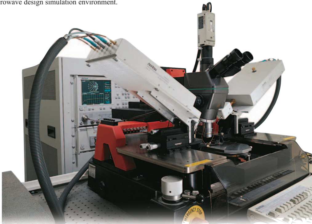
On-wafer Measurements to 500 GHz with the ME7808C
