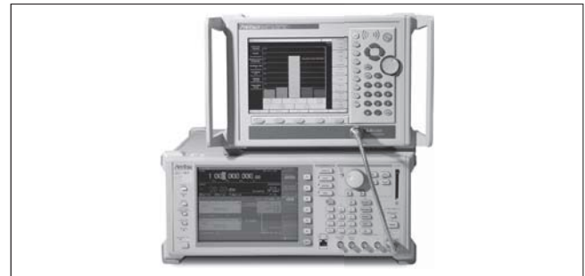
With the companion MG3700A Vector Signal Generator (250 kHz – 3/6 GHz), you get precise test signals with complex modulation matching your wireless system configuration
