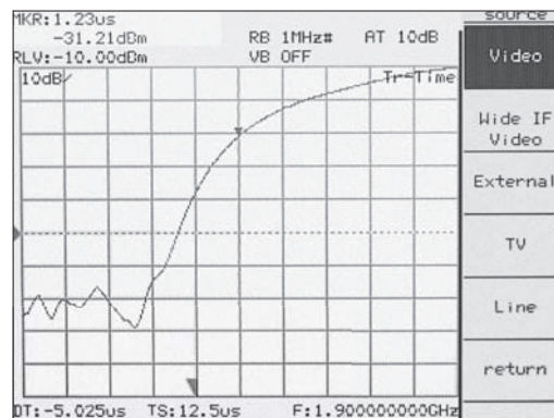
High-speed Time Domain Measurement (TS = 12.5 \mu s)
