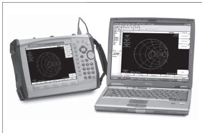
Connect VNA Master to a PC for archiving and additional analysis.
