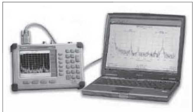
Connect the S8x0D to a PC via a serial (null modem) cable to transfer data or further analyze results.
