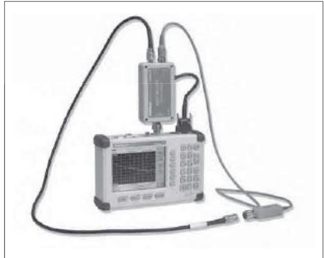
Use 2-port Cable Loss to conduct precise cable measurements of lossy microwave cables.
