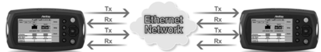
Bidirectional performance test with End-to-End RFC 2544, Two ports simultaneous testing for multiple ports installation.
