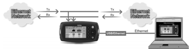
Bidirectional monitoring by dividing both signals and put them into the tester. Two Rxs are used for this application.
