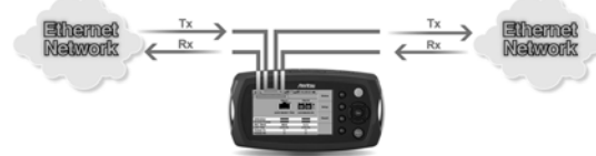
Pass through monitoring by inserting the tester in a network. Tx and Rx of two ports are used for this application.
