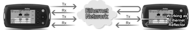
Single end test with Loopback or Using a Ethernet Reflector, Two ports simultaneous testing for multiple ports installation.
