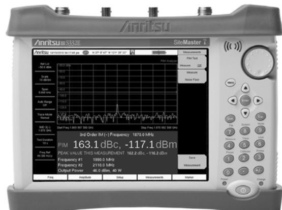
40 W 1900 MHz/2100 MHz Residual PIM Measurement with GPS tagging Listen to relative PIM level with audible tone Save/Recall Setups for standardized testing
