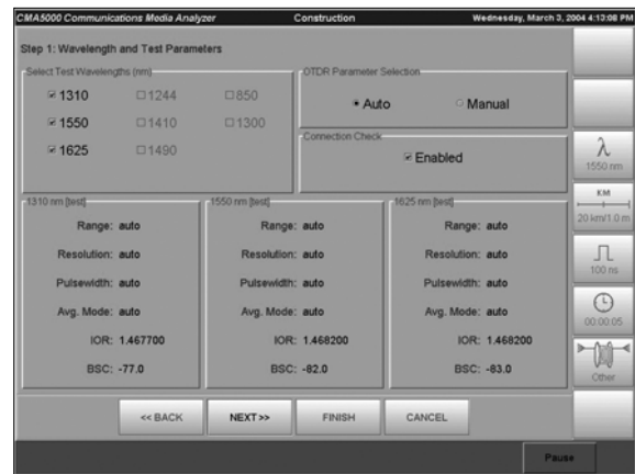
Construction OTDR – automated multi-fiber testing
