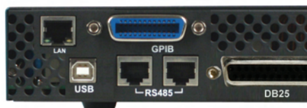
Rear panel of high voltage XLN models
