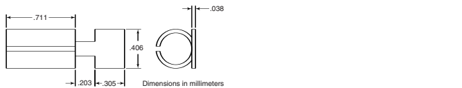
S110-3 Microstrip and Coplaner Waveguide for 0.38 mm glass feedthru center conductor
