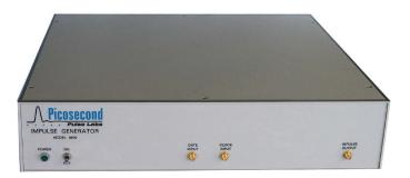
The Model 3600 Impulse Generator produces 7.5-volt, 70 ps duration impulses that are locked to a clock or sine wave input. The added jitter is less than 2 ps. The impulse train can be gated by an external TTL signal. The Model 3600 will function at repetition rates ranging from < 100 Hz to 2.5 GHz.
