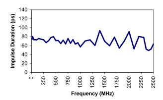
**Figure 4.** Model 3600 Impulse Duration Versus Repetition Rate
