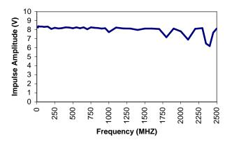
**Figure 3.** Model 3600 Impulse Amplitude Versus Repetition Rate
