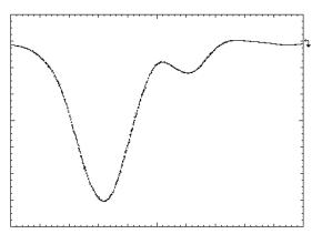
Output with Model 5208 Impulse Forming Network 300 mV/div, 10 ps/div
