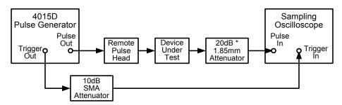
**Time Domain Transmission (TDT) Test Setup**
